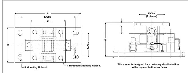
Each comprises base plate assembly, top plate assembly, loading pin and support, bottom pin, mounting posts, retaining clips, earth strap with bolts and washers.
