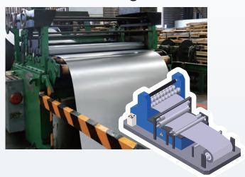
WGC-220 Series devices can be used to numerically check proper loads, improving quality control. Comparators can also be used to set the upper limit and lower limit values for loads, and to transmit a signal and stop the system if an abnormality occurs that deviates from setting values.
