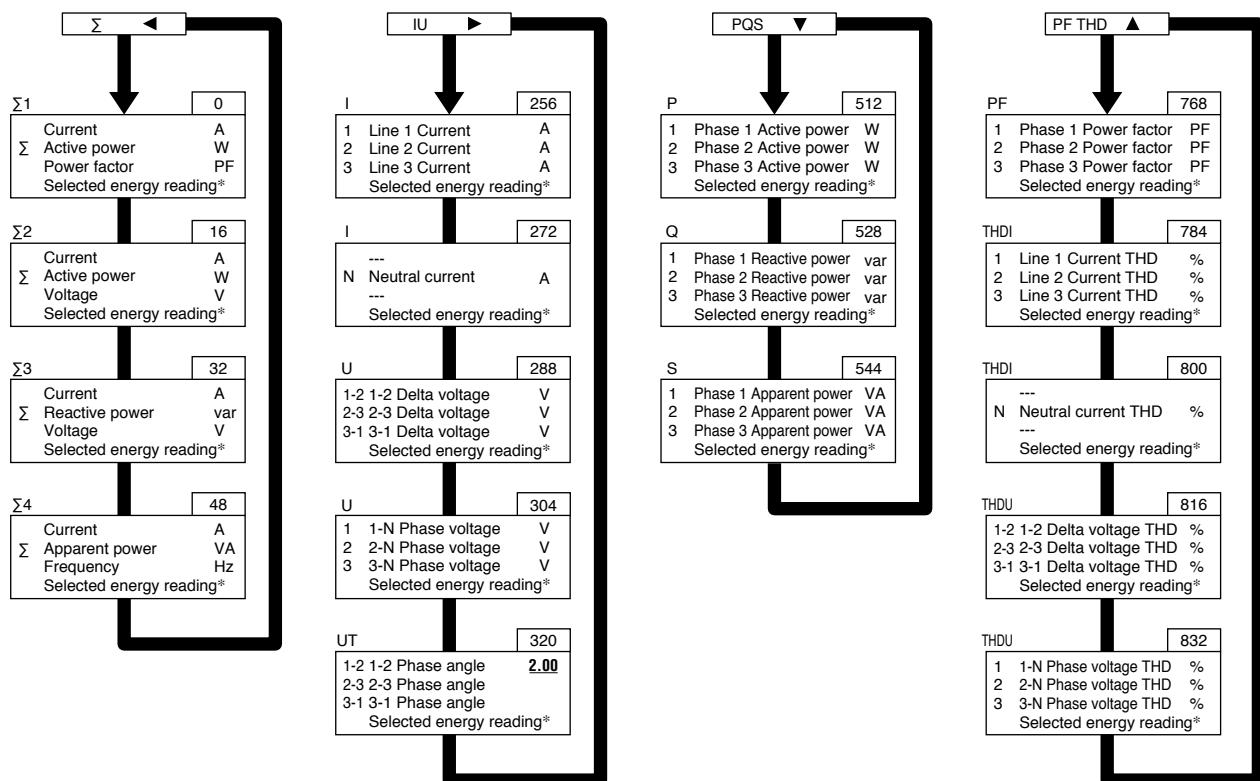
$\Sigma$  thr.  $\Sigma$  views in the above figure shows the factory setting. These combinations can be changed.
