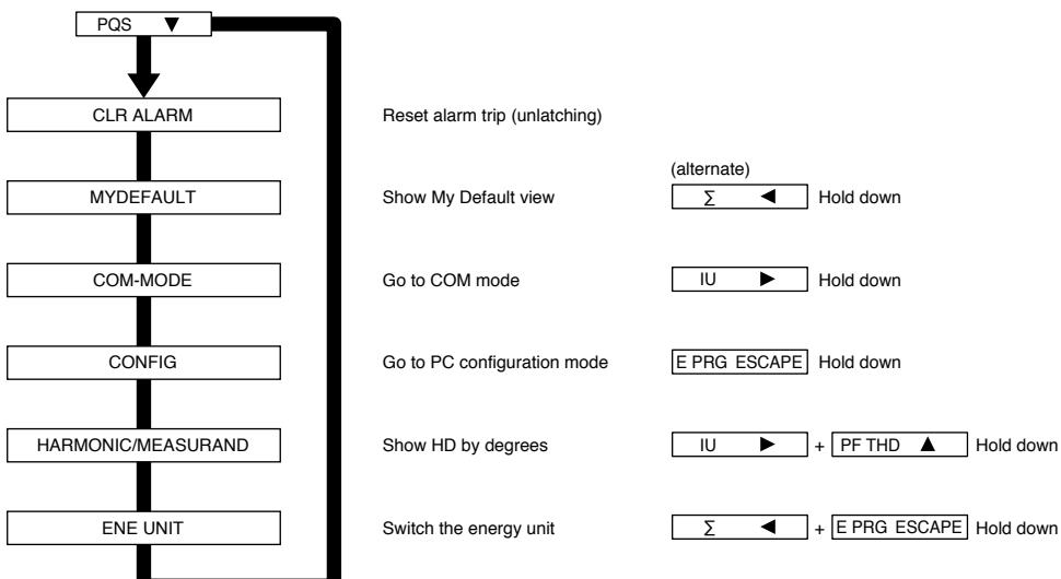
■ HOW TO SWITCH THE DISPLAY FOR LINE 4
