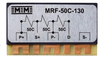
MRF-Series Bridge Completion Modules employ Bulk Metal Foil Resistors. The resistors are specially processed to "match"
