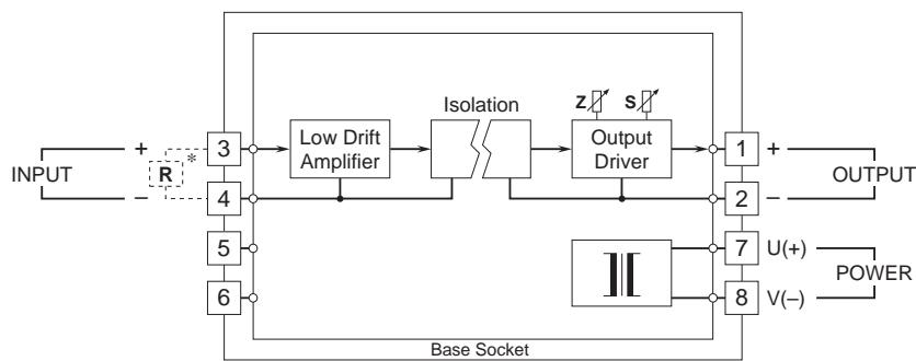
\*Input shunt resistor attached for current input.
