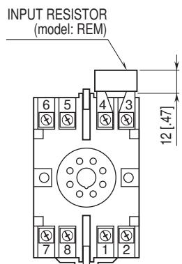
Input shunt resistor attached
