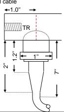
Cable length = 23.6" to 23ft -40°F to 212°F Operating temperature range\* = Maximum static pressure\* 500psi = M5x0.8, 0.43"
