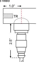
Cable length = 16ft Operating temperature range\* -13°F to 194°F Maximum static pressure\* 145psi M5x0.8, 0.43"
