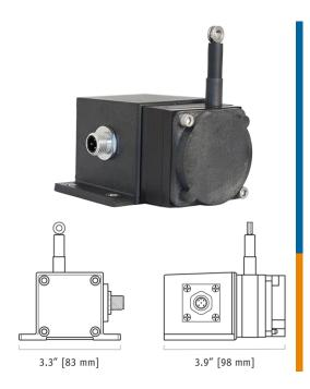
The PT1DN communicates to your PLC over DeviceNET® and provides a precision position feedback signal for full-scale measurement ranges from 2 to 50 inches. Because the PT1DN uses a potentiometer as its sensing element, the position signal is "absolute" and does not have to be reset to a "home" position upon startup.
