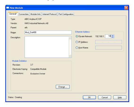
5. Then select inputs and outputs at the same bytes value set on the instrument, see page 36. INTEGER mode.
