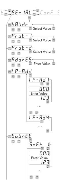
**Modbus:** MODBUS RTU (slave) protocol. used only if PROT-2 is configured equal NONE. See details in the relevant paragraph.
