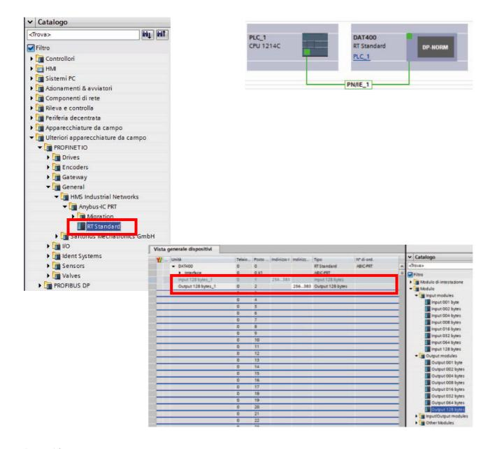
3. Open interface properties and change in the folder IO cycle the value of the number of cycles without updating data. If this value won't be not changed, the cpu will continue to generate communication errors and the module won't recognized on the network, or will continues to give communication errors.
