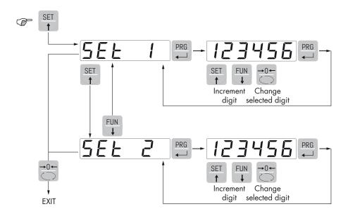
During the step of setting the setpoints, both outputs are disabled. If the setpoint value in memory is 0, the corresponding output is never enabled, regardless of the set-up of the selected setpoints. When the weight is not detectable or out of range, all outputs are disabled (contact open or closed depending on the MODE; see the relevant chapter).
