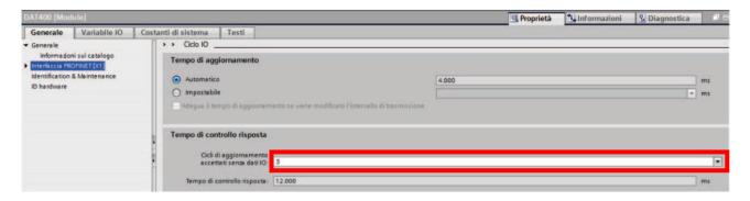
4. Through assigns name to the device, select the module to be parameterized, define in the configuration of DAT 400 the IP address, see PARAMETERS SERIAL OUTPUT. Assign to the module the IP configuration and device name; The device name must be the same as defined in the hardware configuration DEVICE NAME. If the IP address and the NAME UNIT are not defined and equal, the module is not recognized in the profinet network.
