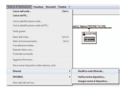
6. Using the Browse button, select the module to be parameterized, define in the DAT 400 configuration the IP address, see PARAMETERS SERIAL OUTPUT. Give to the module the IP configuration and device name. The device name must be the same as defined in the hardware configuration DEVICE NAME; if the IP address and the NAME UNIT are not defined and equal, the module is not recognized in the PROFINET network.
