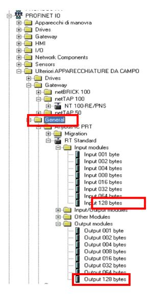
3. Enter inputs and outputs to 128 bytes and associate desired address, define the name of the object eg. DAT400, it will serve for naming the network.
