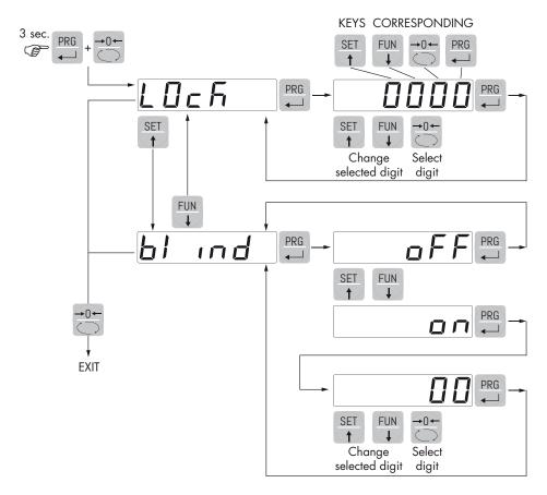
KEYBOARD LOCK/UNLOCK A function that allows you to enable or disable the keys individually. When the keys are locked, the only way to access these settings is to press and hold pressed the PRG + 0 keys for 3 seconds. For more information on the function, refer to the block diagram above.
