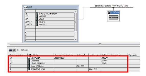
4. Open interface properties and change in the folder IO cycle the value of the number of cycles without updating data. If this value won't be not changed, the cpu will continue to generate communication errors and the module won't recognized on the network, or will continues to give communication errors.
