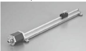
This is the linear profile version of GYSE–R. Between probe and controller, RS–422 differential line driver transmission, providing robustness against electrical noise, is used. In combination with a digital output controller, Min.1  $\mu$  m resolution is possible. The inside probe element can be detached from the outer housing. And by auto calibration function, a difference in the output when you change the probe is adjusted automatically.
