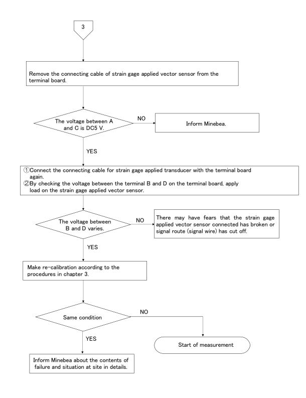
• At the time of checking the voltage between A and C, set the connecting range to DC • V on the measuring instrument such as a tester, or the like.
