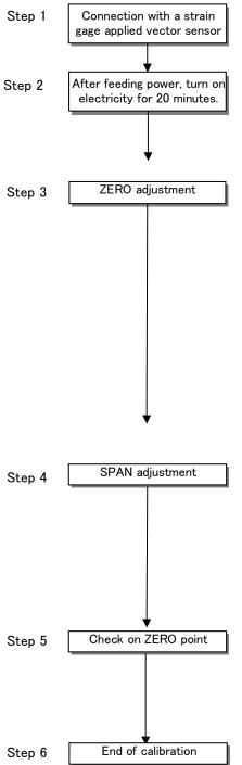
Connect the instrument with a strain gage applied vector sensor.
