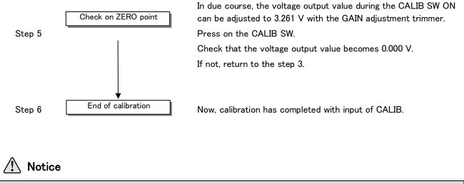
• The rated output value applied to the calculation should be the value that has written on the Test Report individually.
