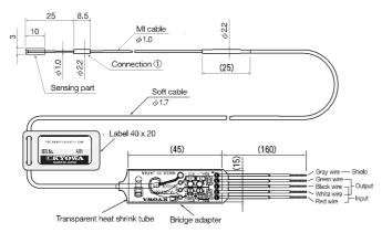
In the case of the gage with no bridge adapter
