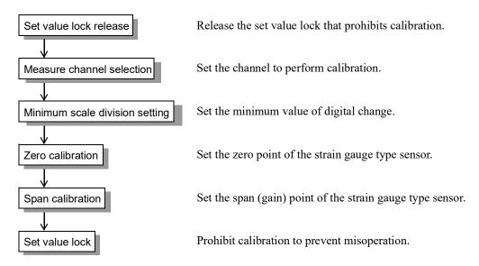
Set value lock release, measure channel selection, minimum scale division setting, and zero calibration are the same as those in equivalent input calibration.
