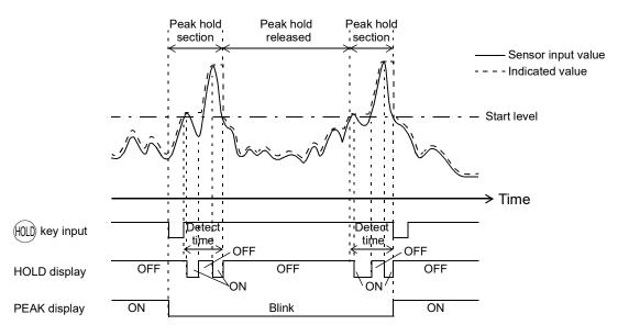
After the (HOLD) key is pressed, when the indicated value exceeds the start level from below it, hold operation starts. After that, the maximum value is held for the set detect time. After a lapse of the detect time, the indicated value and the start level are compared again.
