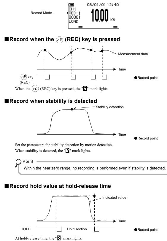
If the hold mode is peak, bottom, or peak-to-peak, and the hold section setting is level or level+time, recording is performed when each hold operation is released (the end level is passed or after a lapse of the detect time).
