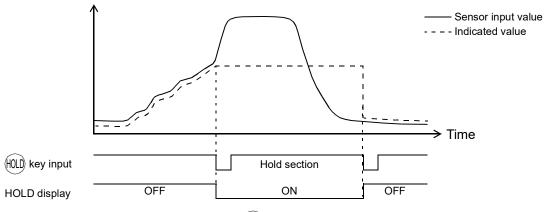
The indicated value of the time when the (HOLD) key is pressed is held. It is released by pressing the (HOLD) key again.
