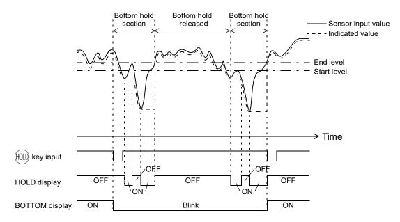
After the (HOLD) key is pressed, when the indicated value falls below the start level from above it, hold operation starts. After that, the minimum value is held until it exceeds the end level. After exceeding the end level, the indicated value and the start level are compared again. The hold operation is stopped by pressing the (HOLD) key again.
