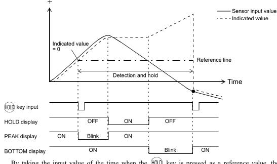
By taking the input value of the time when the (HOLD) key is pressed as a reference value, the maximum difference of the input value is held as an indicated value. The hold operation is stopped by pressing the (HOLD) key again.
