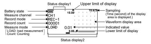
The X-axis and Y-axis widths can be changed by the following operation.
