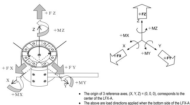
The above are load directions applied when the bottom side of the LFX-A (where cover set screws are located) is fixed.
