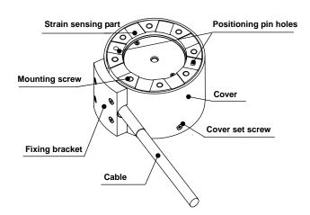
(1)Mounting screw holes Install the LFX-A using the screw holes provided on the top
