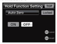
ON: automatically execute the Digital Zero function when a hold starts
