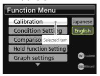
Use the ▲ and ▼ buttons to select the setting item, and press the ENT button to open the setting screen.
