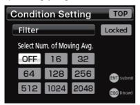
Use the ◀ and ▶ buttons to change the selected option, and press the ENT button. When there are multiple selections, pressing the ▶ button when an option at the right end of a line is selected will select the option at the left end of the next line.
