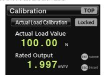
Check the load calibration results. If there are no problems, press the ENT button to confirm them and proceed to the next step.
