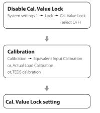
First, we will explain the procedures to be conducted before and after calibration. Then, we will explain the procedures for equivalent input calibration, actual load calibration and TEDS calibration.
