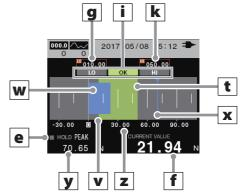
• The indicator value shown on the bar meter screen is the same as the value shown on the indicator value screen.
