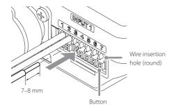
1 Remove 7–8 mm of the covering from the wire being connected, and twist it so that the tip does not come apart.
