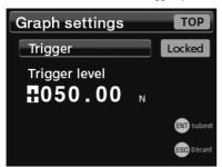
The trigger point is when the indicator value reaches the set trigger level value from the direction set by the trigger polarity.
