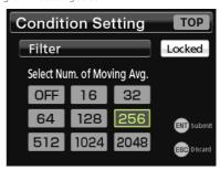
To change a setting value when locked, from the Function Menu, select System settings 1 → Lock, and disable locking for the calibration or setting values (page 34).
