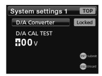
When the D/A CAL TEST screen is open, the voltage value shown on the display is output from the D/A.
