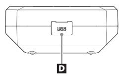
Connector covers are attached to the connectors. Remove the connector covers to use the connectors.
