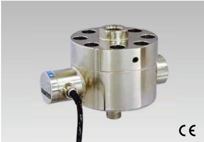
The TLJ-NA Tension Load Cell is designed considering JIS B7721 "Tension/compression testing machines - Verification and calibration of the force-measuring system" and JIS B 7728 "Calibration of force-proving instruments used for the verification of uniaxial testing machine" and is the most suitable for verification of single axis tension testing machine. Calibration in accordance with JIS B 7721 and JIS B 7728 is available at extra cost.
