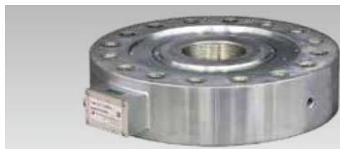
The TCLY-NA is a Tension/Compression Universal Load Cell with low-profile construction and high-capacity. It offers high precision, high output characteristics and an excellent stability because it uses a shear beam for the strain sensing element. This model is widely used in applications like one-axis loading test machine.
