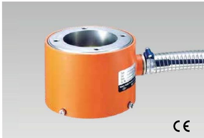
The KCE-NA is a center-hole-type load cell designed to use in tension measurement of anchoring strand. It can deliver stable measurement performance under somewhat eccentric load. An extra model with built-in temperature sensor is available.
