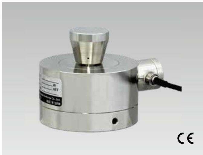
The CLJ-NA is designed considering JIS B 7728 "Calibration of force-proving instruments used for the verification of uniaxial testing machine" and is the most suitable for verification of single axis compression testing machine. Calibration in accordance with JIS B 7728 is available at extra cost.
