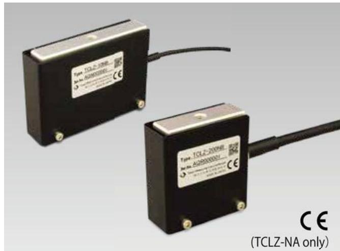
The TCLZ-NA/TCLZ-NB Tension/Compression Universal Load Cell is a high precision load cell that is compact and light weight. With its beam type internal structure, it is widely used as a sensor for controlling industrial machinery.
