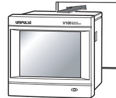
4. Install from the rear the guide rails having been removed from both sides in Step 2, and fix them with the screws (two).
