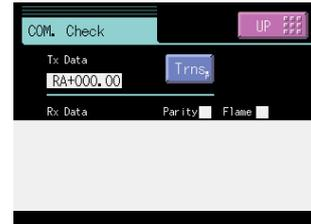
Please transmit something information sentence from connected equipment side to the check on the reception. The data received to "Receive data" is displayed. Please confirm the cable or the setting of communication condition when it is not correctly displayed, when "Parity" or "Frame" lights in red.
