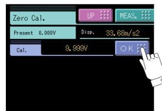
\* The filter by Measure Range in Work Setting is not reflected in the input value on the zero calibration screen.
