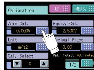
4. Press [OK] button after confirming no-load was applied to the sensor.
