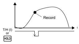
In addition, when using hold with SI/F print at hold value, the value is recorded at the time of release.
