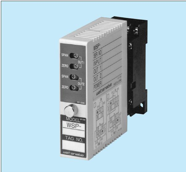
This compact plug-in signal converter with two insulated outputs converts the secondary outputs of PTs (VTs) in power substations, motor circuits, etc. into instrumentation signals. Since Type PTEW adopts the true root-mean-square value operation system, it ensures particularly high reliability against distorted waves.
