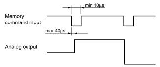
\* For memory command, input print command signal from a connected external counter.
