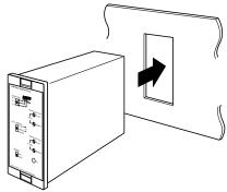
② Mount the panel fixture which is supplied with this instrument from rear side of the instrument, and tighten the mounting screw.
