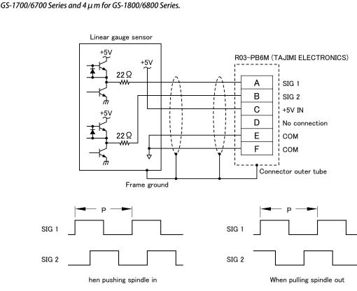
P=40  $\mu$  m : GS-1700/6700 Series P=4  $\mu$  m : GS-1800/6800 Series When replacing the gauge head of GS-1700/1800/6700/6800 Series Linear Gauge Sensor, take care not to give twisting force exceeding 0.3Nom to the spindle. (For details, see "Replacing Gauge Head.")
