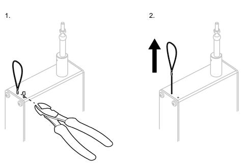
Transport protection (for some sensor models) prevents the measuring cable from being extracted before mounting the sensor. Only remove immediately before mounting:
