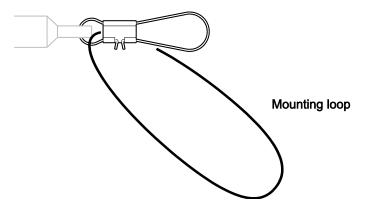
For example, fit a mounting loop and put it around your wrist. Do not remove the mounting loop until after final installation.
