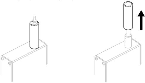
The kink protection prevents the cable fixing from buckling and damaging the cable. Remove in the direction of the cable.
