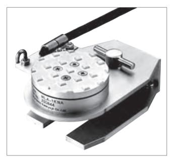
The Pedal Force Transducer, which is a load cell to measure the pressure applied to the passenger car's brake pedal, can be installed easily without modifying the pedal. Cables do not break easily even when handled roughly.
