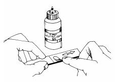
Now apply a liberal amount of M-Prep Neutralizer 5A and scrub with a cotton-tipped applicator. With a single, slow wiping motion of a gauze sponge, carefully dry this surface. Do not wipe back and forth because this may allow contaminants to be redeposited.
