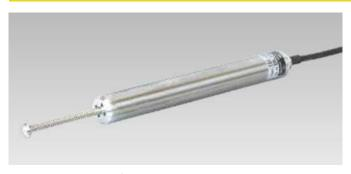
FDP-A series is a DC operated LVDT which can be measured with not only our TDS series data loggers but DC excitation type dynamic strainmeters and handheld strainmeters. In addition to high output and high response, waterproof structure and all stainless steel made external parts make underwater measurement possible.
